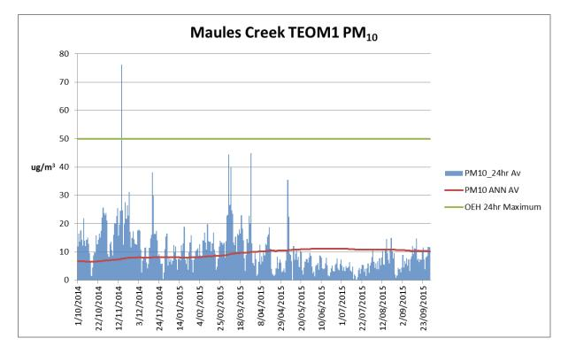
TEOM Figures – Particulate Matter PM<sub>10µg/m3</sub> and PM<sub>2.5µg/m3</sub>
